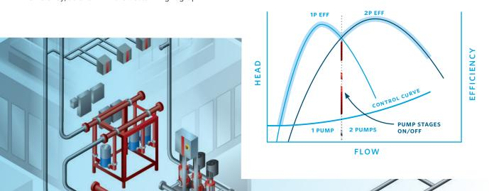
Because HVAC pumping systems mostly operate at partload, a design using two or more smaller pumps is more efficient than one larger pump. In a two-pump system, if one pump fails, the remaining pump can serve the system requirements with up to 70% flow redundancy. The capacity split can be adjusted based on the building type and duty requirement.
